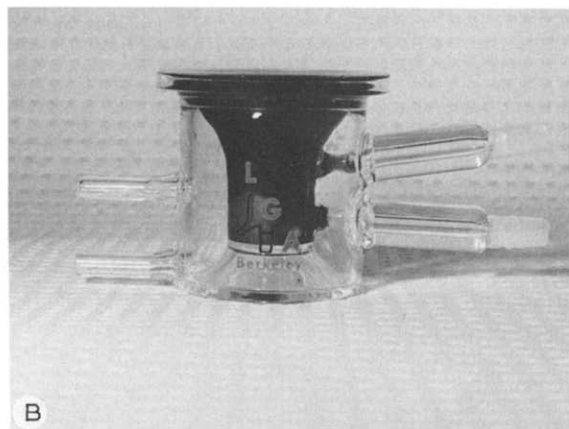
Fig. 3. A: a "GH" flow-through diffusion cell for use with hairless mouse skin. Complete and instantaneous (< 30 s) stirring of the receptor phase is seen. (The top of the cell has been removed for photography.) B: a "GH" flow-through diffusion cell for use with full thickness guinea pig skin. The gradual increase in the diameter of the receptor compartment achieved with the funnel design gives complete and instantaneous (< 30 s) stirring. (The top of the cell has been removed for photography).
