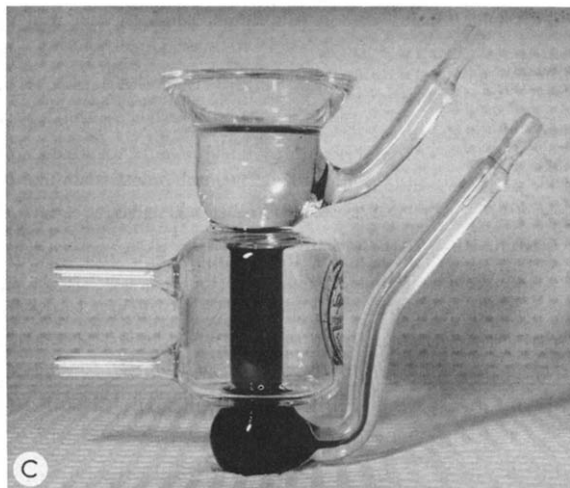
Fig. 1. Franz-type diffusion cells (A, B, C). Subtle differences in construction result in large variations in receptor phase stirring of the upper portion of the cells. Volumes = 11 ml; 9.7 ml; and 11.5 ml (left to right). The top of the cell has been removed for photography.
